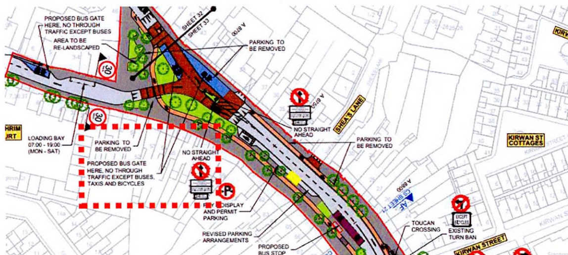
Figure 7.0 Extract from Sheet 33 of the General Arrangement drawing illustrating the proposed bus gate (red dashed line) at the junction of Prussia Street and Aughrim Street.
